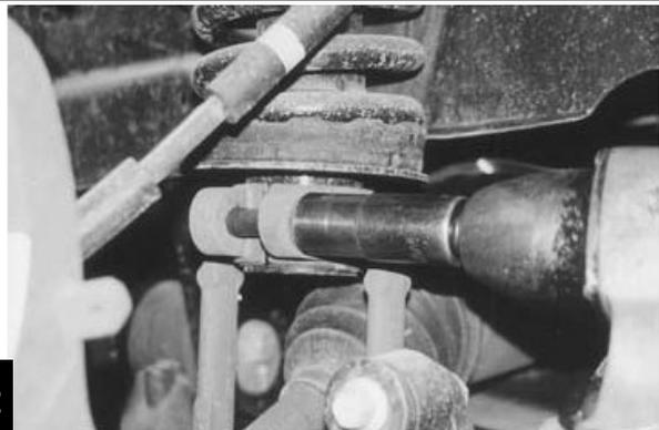
With the bolts removed from the fork, there is enough room to drop the strut from original position. A pry bar is helpful to separate the fork from the bottom of the strut assembly.
