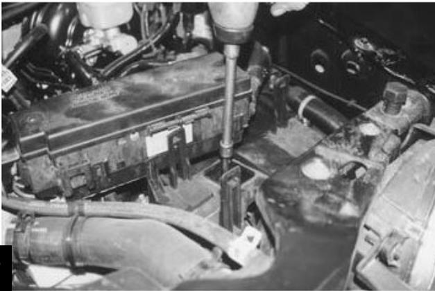
The connectors that attach the wires to the tray can be easily disconnected. Disconnect the battery sensor from the bottom of the battery tray.
