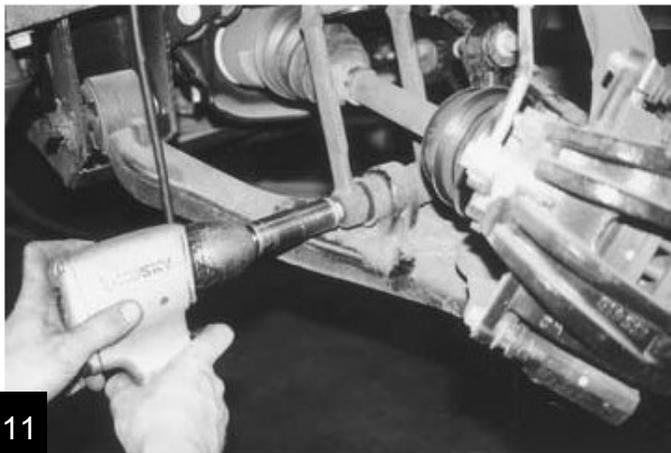
Use a 21 mm socket to remove the bolt that secures the top of the fork to the bottom of the strut assembly.
