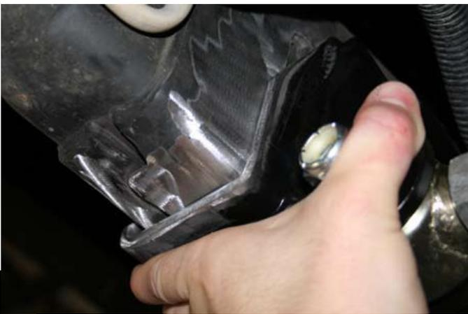
With the brace bar removed, final weld the frame bracket as well as the drop bracket at the steering box.
