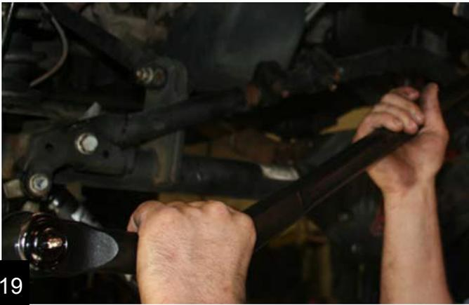
Reinstall and torque the wheels and tires to 95-115 ft-lbs. Lower the Jeep and do a quick track bar adjustment. The axles should be centered under the vehicle. Torque the adjustment sleeve bolts to 26 ft-lbs.
