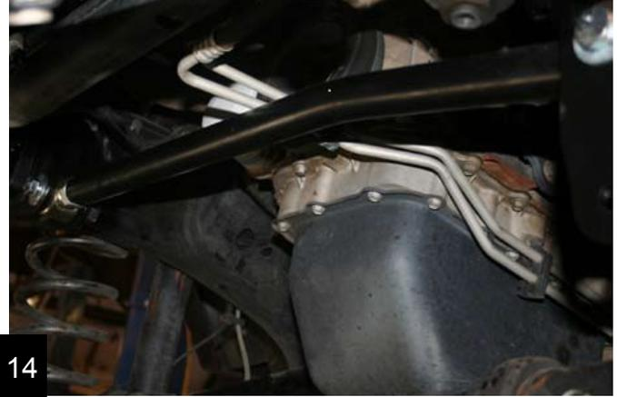
Using a 13/16" drill bit, drill out the knuckle and tap the new taper sleeve in from the top. Be sure to drill straight.
