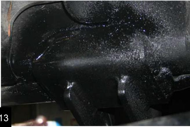
Reinstall the brace using the supplied hardware. The 3.5" bolt is used in the drop bracket and the 3" is used in the frame brace bracket side. Tighten the jam nut with an 1 1/4".
