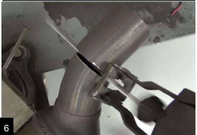
Use a grinder and clean up the cut ends of the exhaust pipe.
