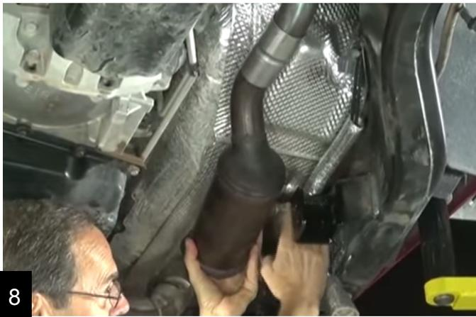
If the converter is properly oriented, the O2 sensor will be easy to remove and clear the new control arm bracket. With all clearances checked, weld in place.
